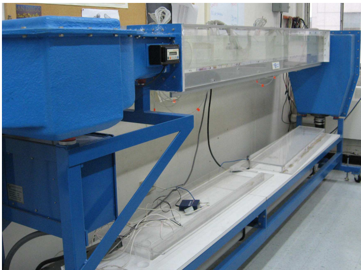
Figure 3: Water tunnel housed in the Dynamical Systems Laboratory.
